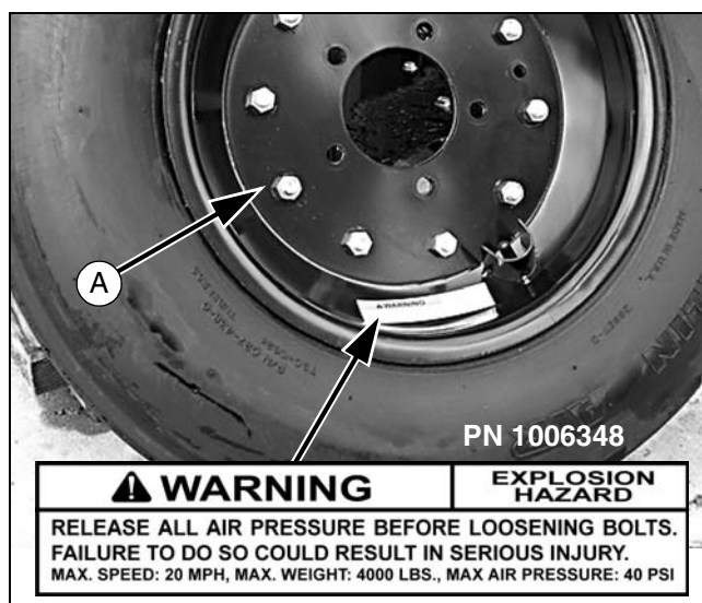
Figure 23. Split Rim Tire Servicing
